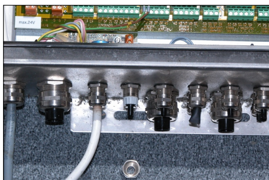
1. Remove the top of a free cable gland
