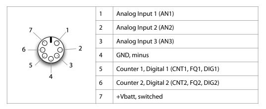
The power to sensors is supplied on pin 7 (+Vbatt) before the sensors are sampled. The time elapsed between applying power and the actual sensor sampling is set to 2 seconds by default, but it can be changed (see the XGV command). All input sensors must be referenced to the ground pin (pin 4). Keep the analog input cables short and always use only shielded cable! The maximum recommended cable length is 10 meter.
