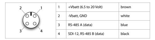
Notes: The colors in the last column are valid for the standard cable delivered with the device. Pin 3 is not used in SDI-12 mode.
