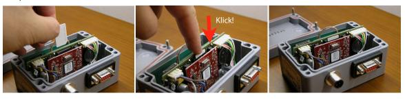
4. Now remount the cover on the housing again. Please make sure that the seal stays in the intended guide trench of the cover and does not step out. Now screw the 4 scews with moderate power back to close the housing.
