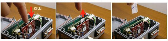
3. Insert now the new card into the card holder, please make sure that the card is inserted with the correct side (see picture). When the card is latched you should feel the same "Klick" as when removing the other card, the new card now sits in the card holder.
