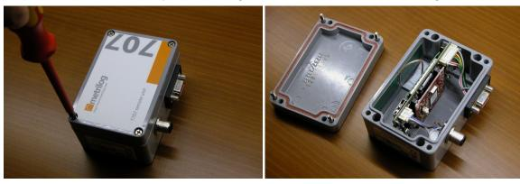
2. Identify the SIM card as shown on the photo. Slightly push the card down, until you can feel a "Klick", that indicates the release the SIM. The card now sticks out a bit and can be removed.
